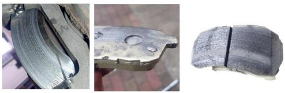
**Case Study:** An end-user complained a pad destroyed the disc surface within 1000km. The shim of the inner pad is gone. Pips/lugs on backing plates are squashed.
