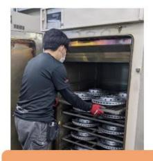
The heat treatment does not directly improve friction coefficient, but reduce the risks of distortion and crack.
